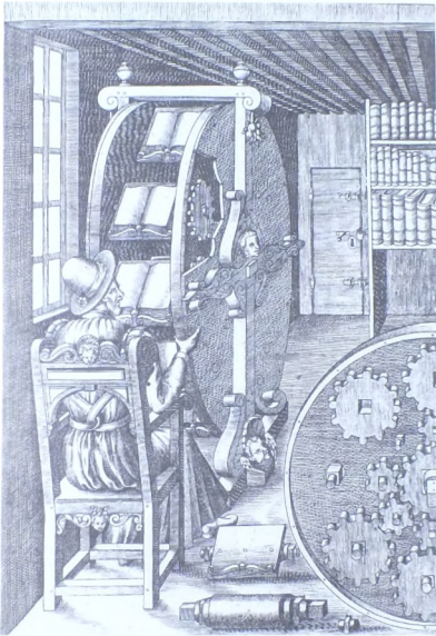
Figure 3. The book wheel from Agostino Ramelli's Le Diverse et artificiose machine (1588).
